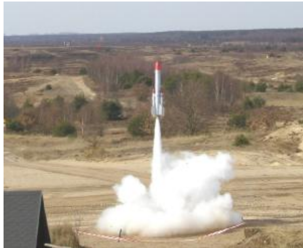
Launch of the reusable hot water rocket B4-1
